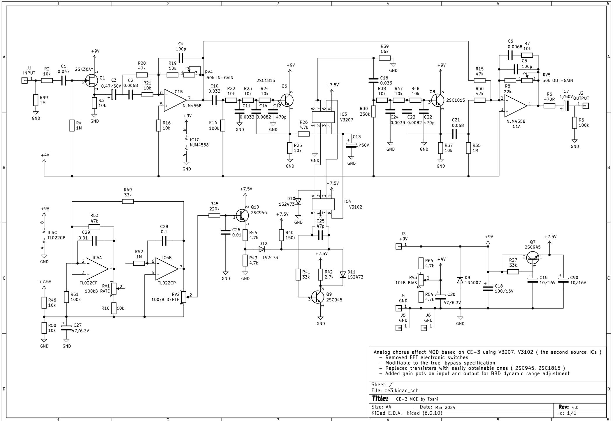
Analog chorus effect MOD based on CE-3 using V3207, V3102 ( the second source ICs )
