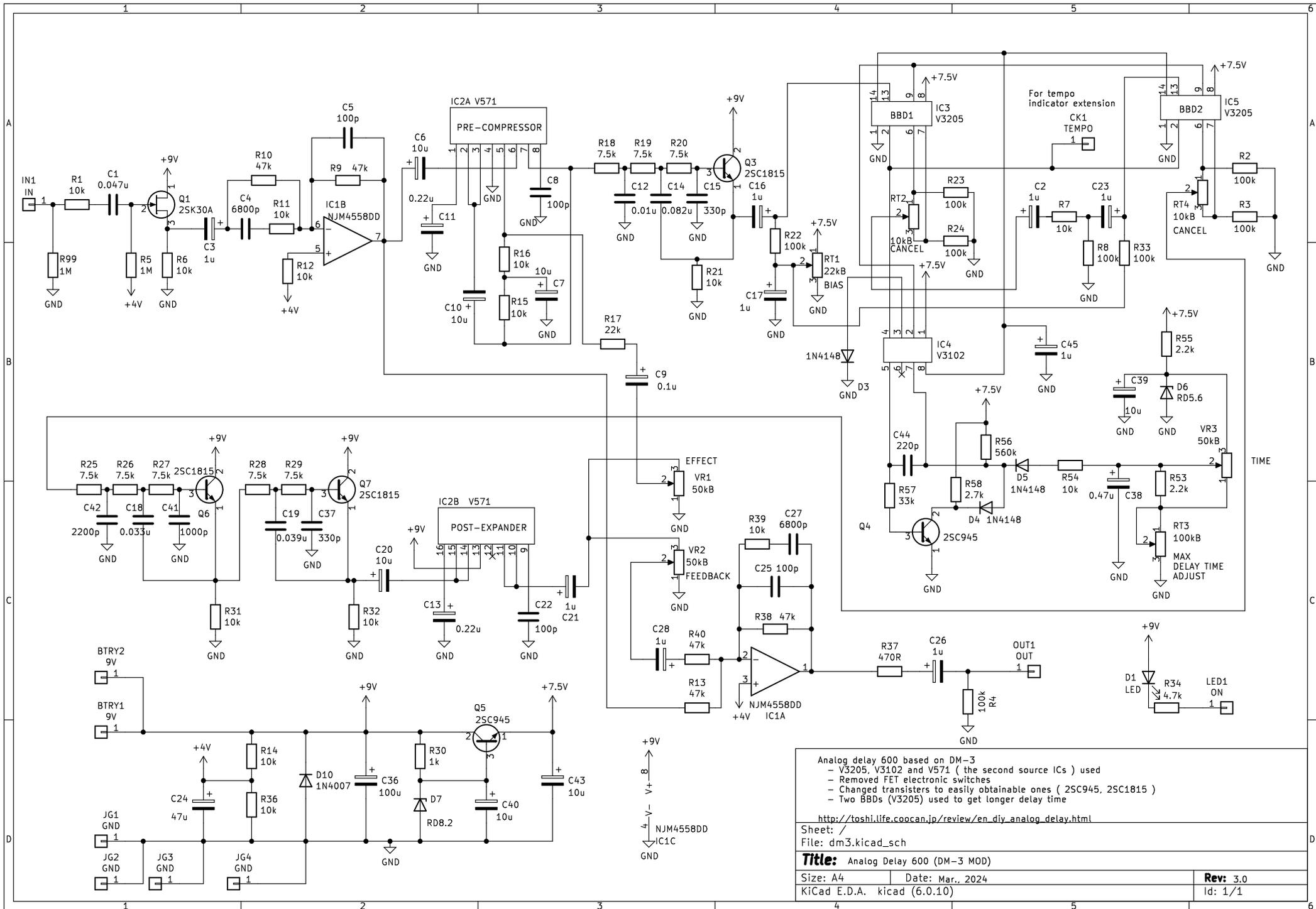
Analog delay 600 based on DM-3
